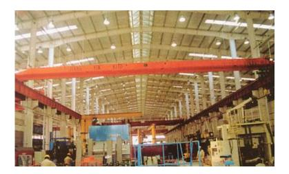
LHBJ explosion proof electric hoist bridge cranes are designed adopting Japanese technology. Their working grade are between A3-A5, lifting capacities are from 1t-20t, spans are 10.5m-25.5m. They are suitable for the explosive environment where the temperature is from T1-T4 and is full of flammable gas or the explosive mixture of steam and gas.
