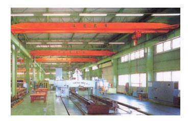
LDA cranes are suitable for hoisting, handing and ransporting weights in machine shops and stores, etc. Operation mathod:floor control, cab control.
