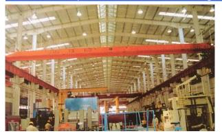
LBJ explosion proof electric single-girder cranes are light and small. Their working grade are between A3-A5, lifting capacities are from 1t-10t, spans are 7.5m-22.5m. They are suitable for the explosive environment where the temperature is from T1-T4 and is full of flammable gas or the explosive mixture of steam and gas.
