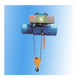
Operating principle of frequency conversion electric hoist is that the univertor controls the speed of the motor through changing the power frequency. The feature of it is the following: Decreasing the impact of starting and stop
